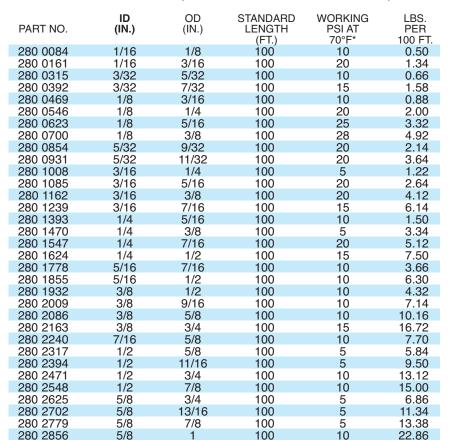
Add length suffix to part number when ordering. Example: 100 ft. of 1/16" I.D. x 1/8" O.D. tubing is part number 280 0084-100.
